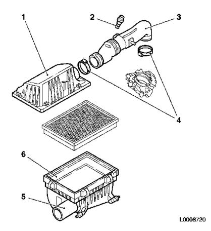
**Important:** Prior to installation, clean any contamination (grease, oil etc.) from the air intake pipe and the connection pieces.
